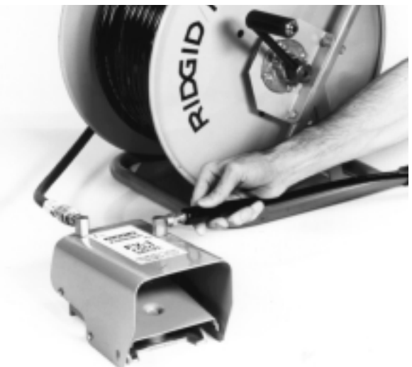
Figure 8 – Foot Valve Connection
