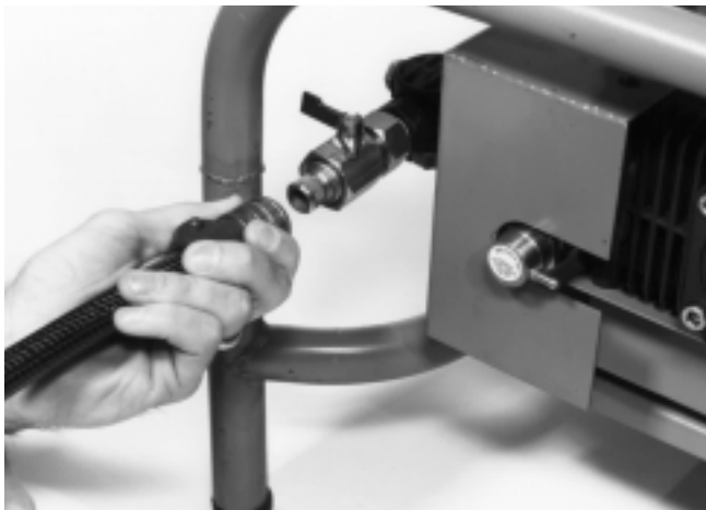
Figure 4 – Connect water supply hose to jetter. Close inlet supply valve (shown in CLOSED position)
